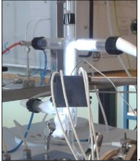
Figure 8 - Plasma generation across a packed-bed reactor.
