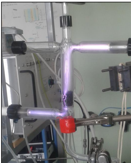
Figure 28 – Plasma-assisted reaction in the packed-bed reactor with formation of micro-discharges across the catalyst.
